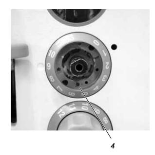
Depending on the sewing equipment used, the stitch length setting has to be limited to 6, 9 or 12 mm.  $\ensuremath{\text{\textbf{GB}}}$
