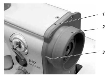
The handwheel 2 has graduation printed on it.
