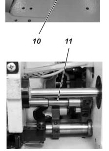
The shaft 11 is fixed on surface in the positioning frame 14 at position 3 with two screws in series.
